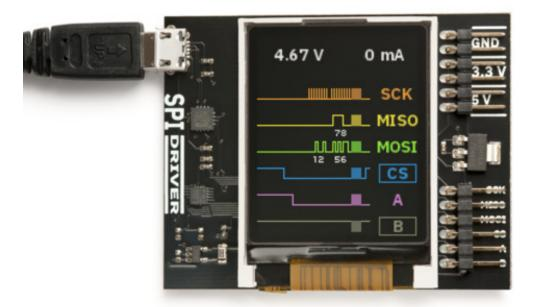
SPIDriver is an easy-to-use, open source tool for controlling SPI devices over USB. It works with Windows, Mac, and Linux, and has a built-in color screen that shows a live "dashboard" of all the SPI activity.
